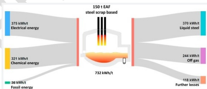
Figure 1: Sankey flow diagram of EAF energies, acc. to [10]
