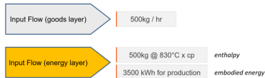
Figure 4: Usage of the energy flow layer for different mass-related energy types
