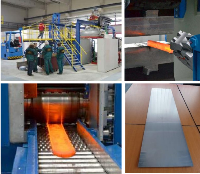
Figure 7: 500 kg vacuum melting (1), automated open die forging (2), hot/cold rolling in 2/4 high, reversing mill (3), final cold rolled sheets (4)
